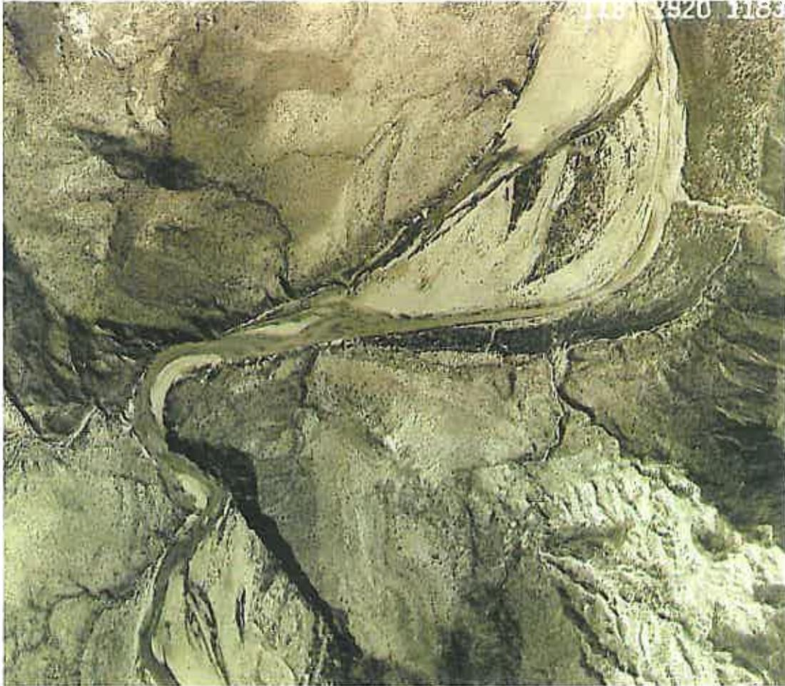
Figure 20. Verde River at Horseshoe Dam site (T7N, R6E, Sec 2). 1934 aerial photograph showing braided channel pattern and constriction, as a result of geologic control. Note that channel occupies entire width of valley.
