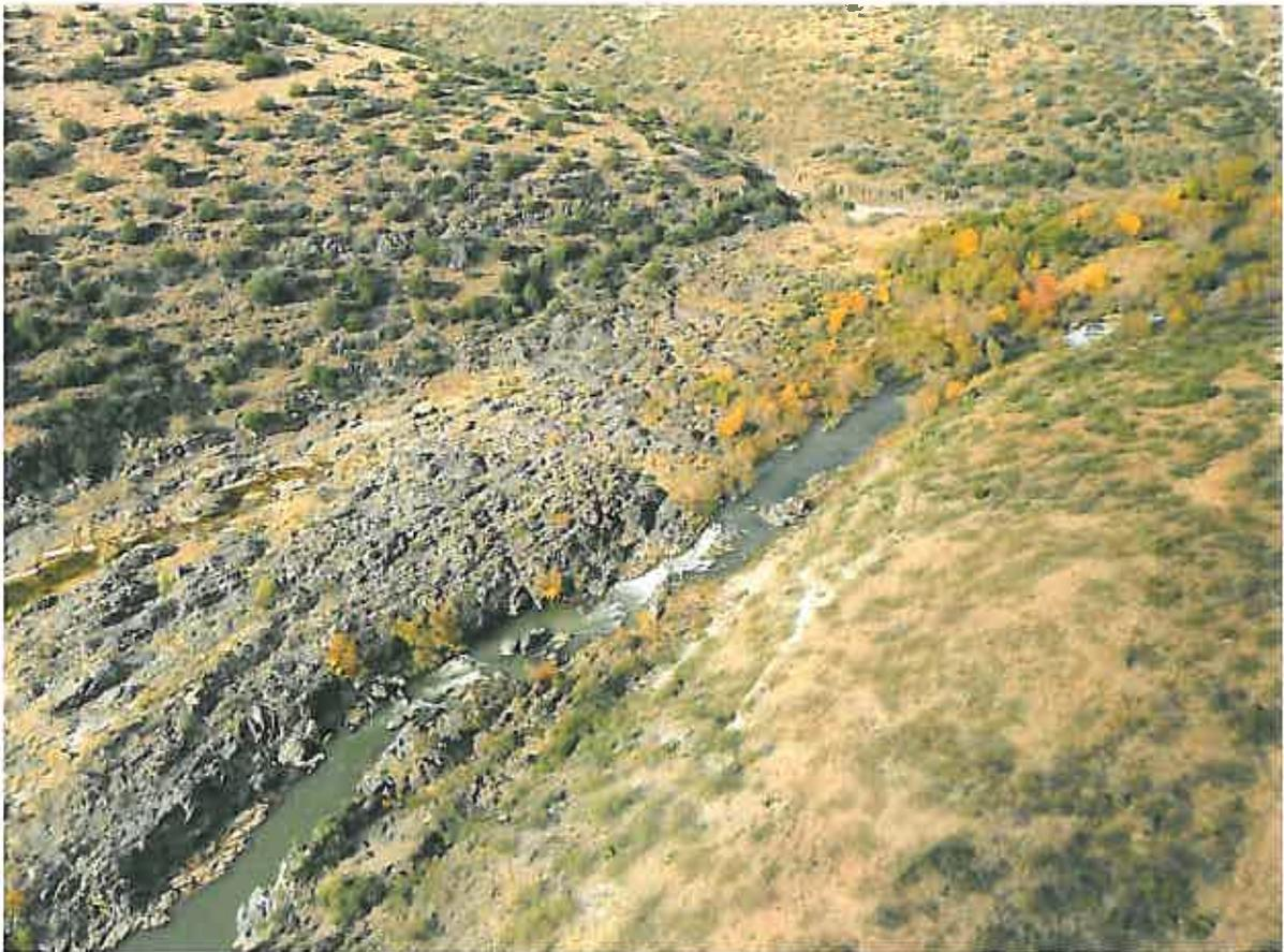
Figure 3. Verde River in the vicinity of Verde Falls and Pre-falls. Bedrock forms bed and banks of channel. Drop across the falls in the center of the photo is about 4 feet. (Photo by R. Mussetter, October 2013)
