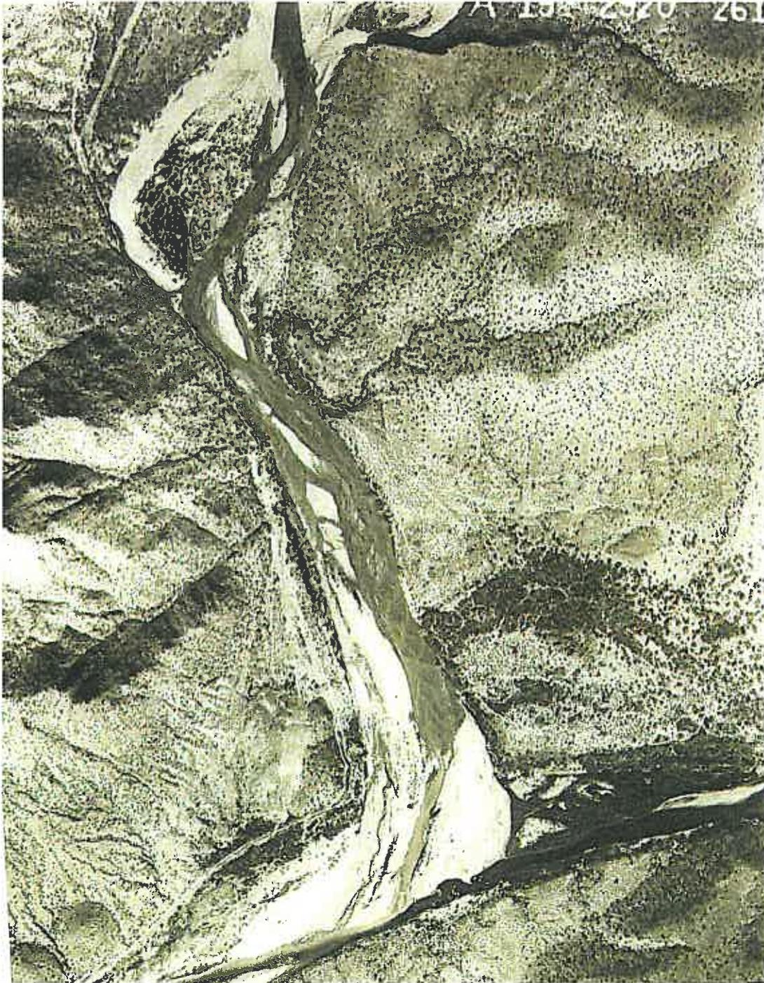
Figure 22. Verde and Salt River confluence (T2N, R7E, Sec 5). 1934 aerial photograph showing braided channel pattern and constriction. Note that large sediment delivery from Verde River forces Salt River channel to south side of valley.
