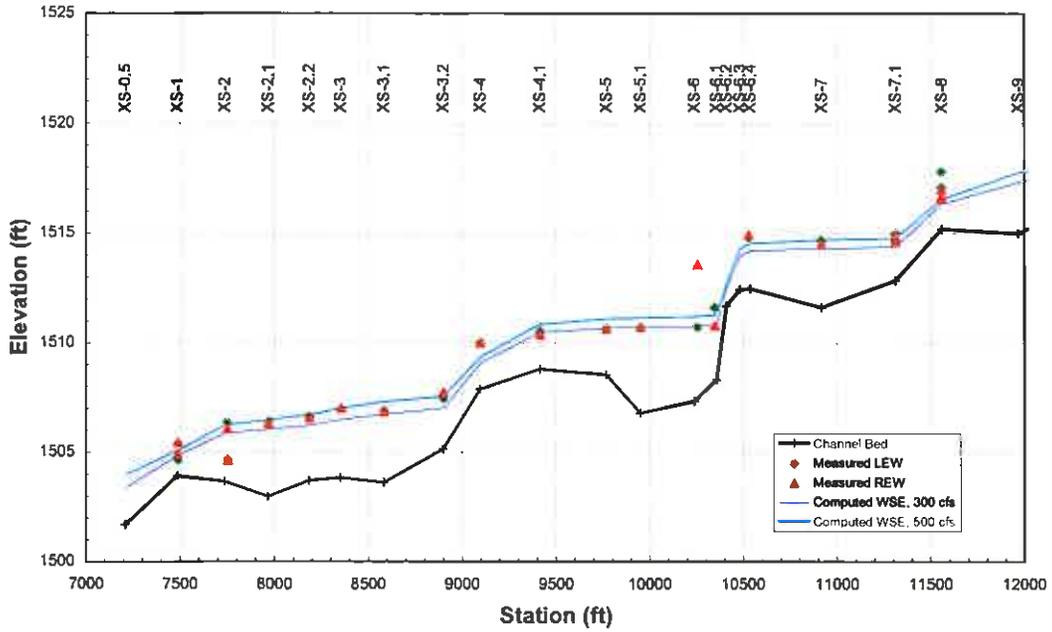
Figure 30. Site 3 surveyed water-surface elevations and computed water-surface profiles for the discharges at the time of the survey (300 to 500 cfs).
