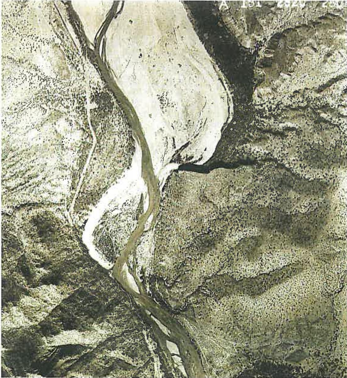
Figure 21. Verde River at “bottom of Fort McDowell Indian Reservation” (T3N, R7E, Sec 31). 1934 aerial photograph showing braided channel pattern and constriction, as a result of geologic control. Note that the channel occupies the entire width of the valley.
