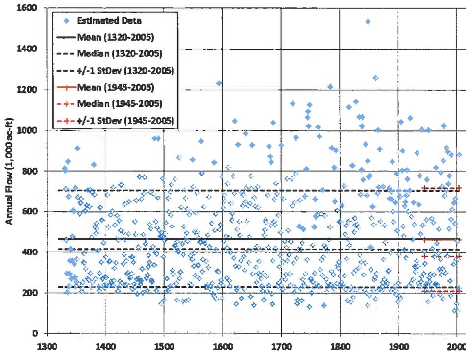
Figure 10. Estimated annual flow volumes from 1320 to 2005, based on tree ring analysis (Meko and Hirschboeck, 2008). Also shown are the mean, median and  $\pm 1$  standard deviation for the full period and the period that overlaps with the available records at the *below Tangle Creek* gage.
